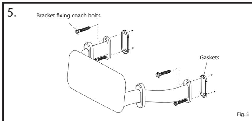
Fit Gaskets onto wall fixing plate as shown in Fig 5.
