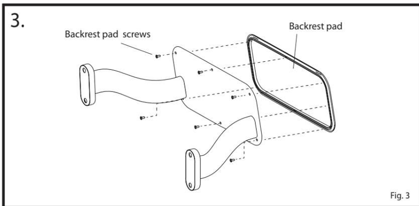
Attach backrest pad using 6 x backrest pad screws as shown in Fig. 3. Ensure all screws are started before tightening. Do not overtighten.
