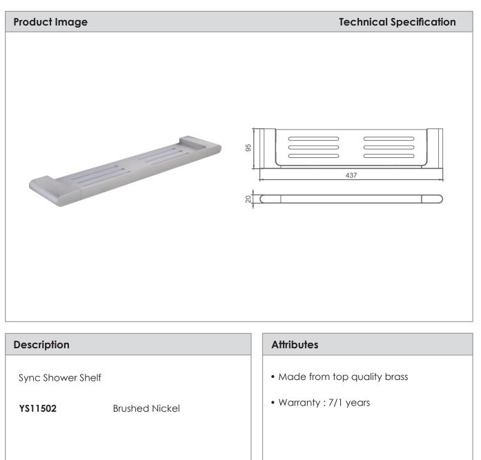
\*All dimensions are in millimeters and are subject to normal manufacturing variations. Actual dimensions should be checked prior to installation. Yushi pursues a policy of continuing improvement in design and performance of its products. The right is therefore reserved to vary specifications without notice.
