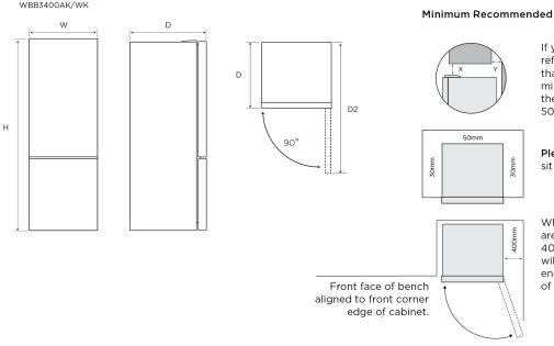
If you have a cupboard above the refrigerator with a rear gap of less than 100mm (Y), recommended minimum clearance at the top of the refrigerator increases from 50mm to 100mm (X).
