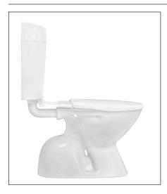
The Uniset 2 is a mid sized modern styled cistern designed for retrofit installations. The Uniset 2 cistern is a two button, dual flush integrated system comprising of cistern, seat and flush fitting connection plate which conceals the flush pipe and water connection. This versatile 6/3 litre dual flush cistern can be converted to 4.5/3 and 9/4.5 litre with the benefit that the matched suites are suitable for multi purpose applications and can be used where authorised for septic installations.
