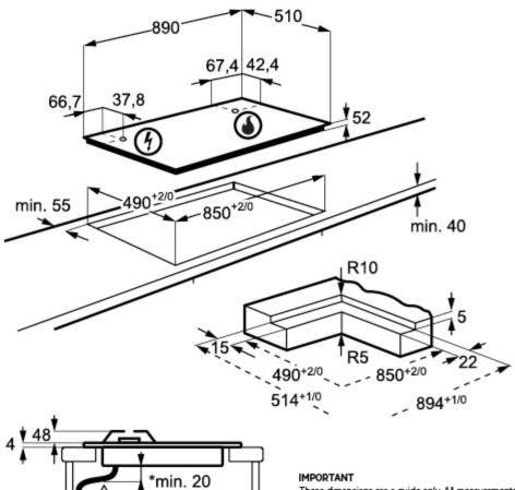
These dimensions are a guide only. All measurements are in millimetres (mm). For complete installation instructions, refer to the manual provided with product.
